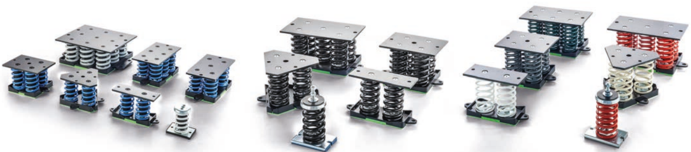
AMC Max.Deflection: 25mm. Nat. Frequency: 4Hz
